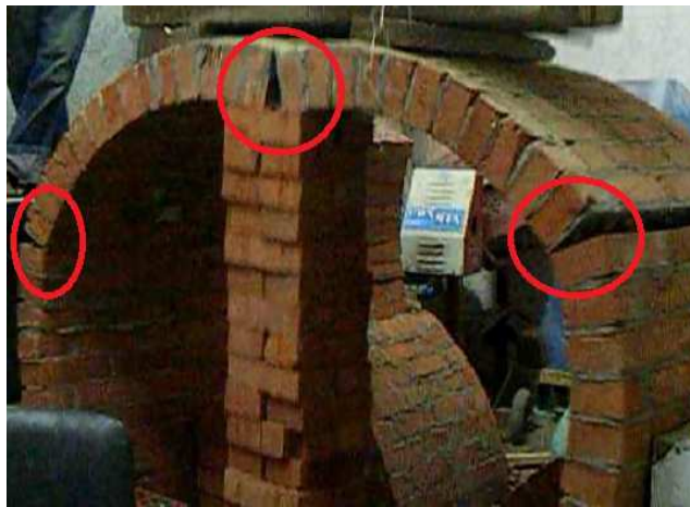
Figure 10 Control masonry vaults failure pattern.
