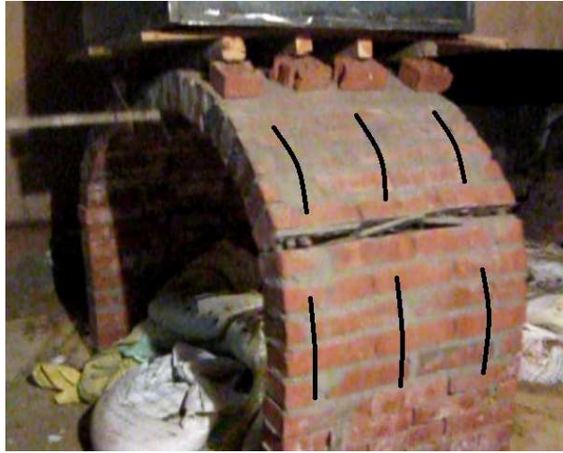
Figure 14: Mode of failure for vaults strengthened by steel reinforcement
