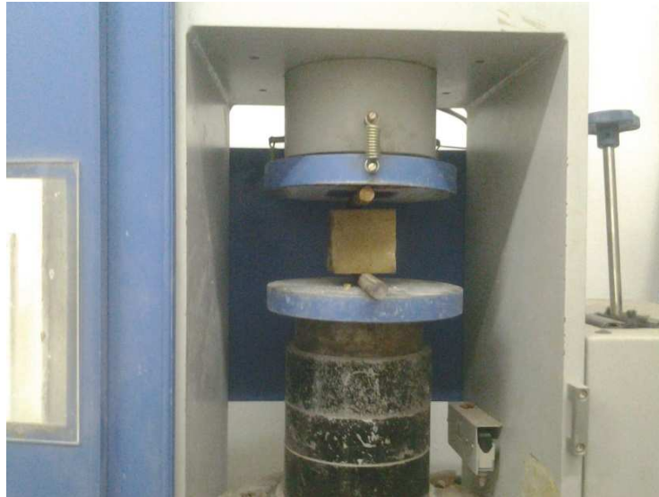
Figure 5: Polyester Mortar cubes for indirect tension testing, 70x70x70 mm, [11].
