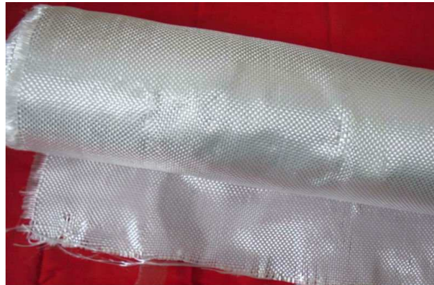
Figure 3: FRP roving 600 sheets
