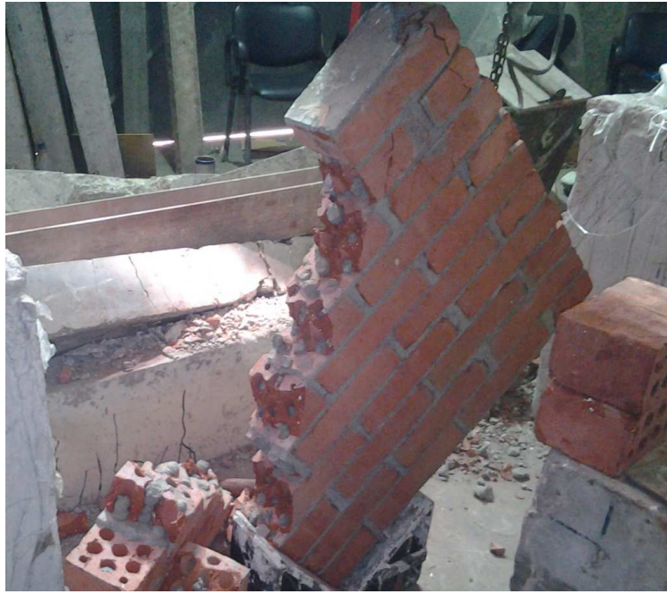
Figure 6: Failure mode for Control wallets.
